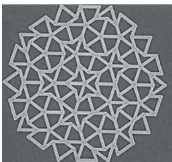
Interconnected permalloy nanobars (bright) with two different lengths of 500 and 800 nm forming an artificial two-dimensional quasicrystal on a nonmagnetic substrate (dark). (V. Bhat et al., unpublished)
